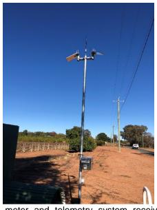
The new meter and telemetry system receives minor upgrades such as the double solar panels (pictured above)
