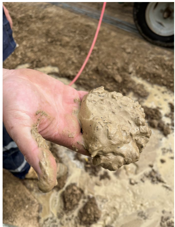
Example of piezometer desilting in progress. This piezometer was previously 'dry', it is now 2M deeper. Will be checked for reading in 2 weeks.
